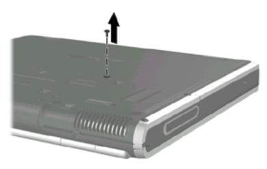
Removing the hard drive retaining screw
